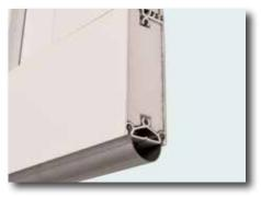
The bottom weather seal keeps out wind, rain, debris and other elements. Optional 3-layer sandwich construction with insulating polystyrene core increases energy savings (R-value 5.6)
